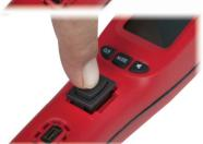
Position the new Rocker Switch into the switch cavity and carefully press straight down until the switch is flush with the housing.
