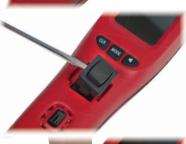
Carefully remove the Rocker Switch with an appropriate pry tool or small screwdriver. Do not apply excessive force.
