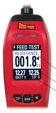
**FFEED TEST** - Power Feed Test (PFT) is used to check resistance on static circuits or voltage drops on active circuits by simply probing one connection of the circuit being tested.
