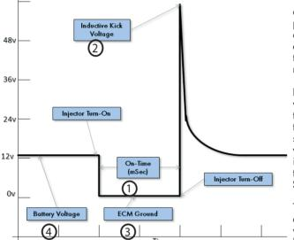
This is displaying a single injector pulse. The vertical axis represents the circuit voltage and the horizontal axis represents time.
