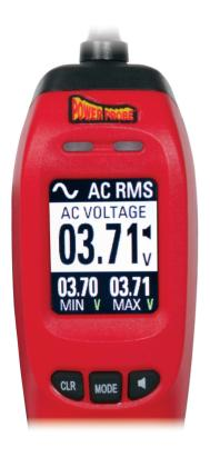
◆ AC RMS mode is for measuring AC (alternating current) voltages and can be used on any AC voltage or pulsed waveform signal where an RMS averaged voltage measurement is required.
