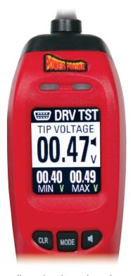
DRV TST = Driver Test Mode is design to test the drivers (transistor) inside the module's (PCM, BCM, GEM, etc.) control circuit.
